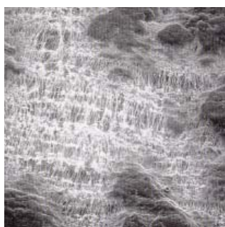
Media filtrant SINBRAN® filtration de surface surface lisse structure fine
