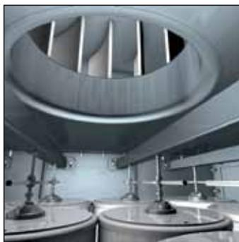
As an alternative to the integrated fan section, an external fan can be installed for the simultaneous operation of several AERO® separation systems at once. This may also be necessary for single systems, depending on the location of the application and
