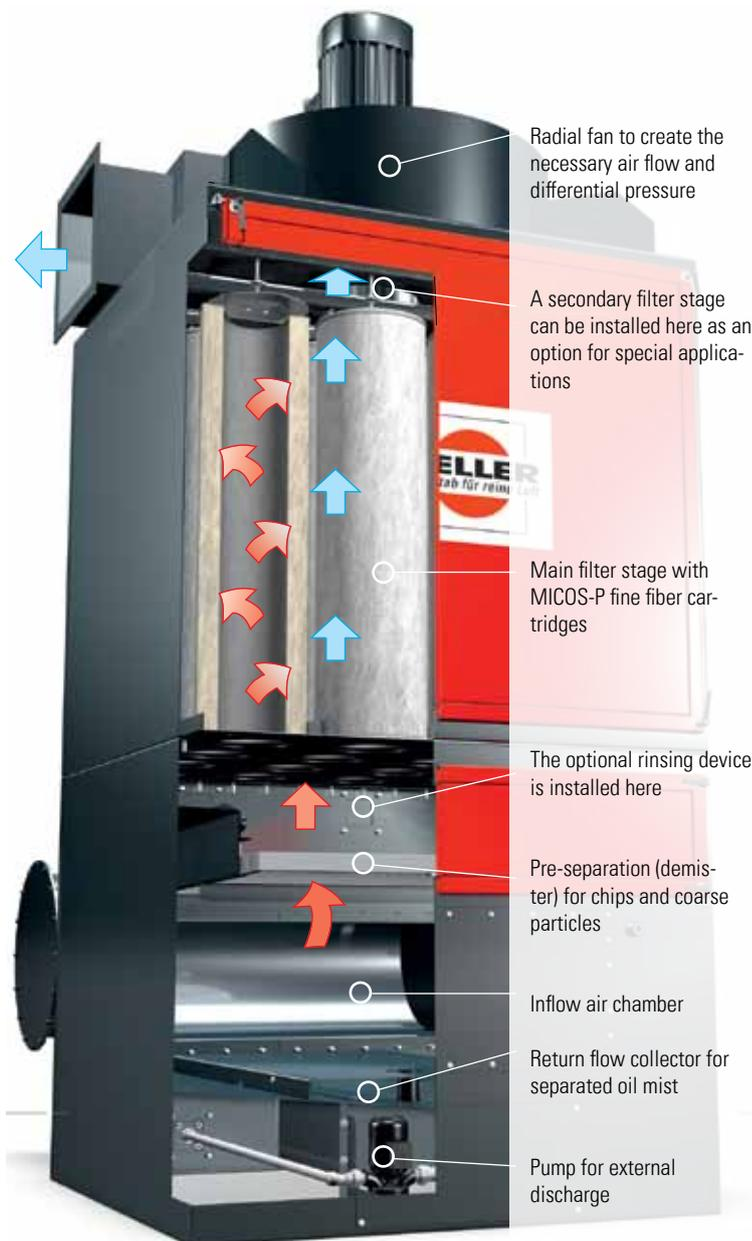
AERO® oil mist separator for coolant aerosols, size 3
